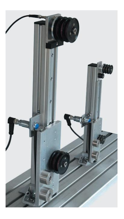
Uhing Tension Control is a dancer system that helps control line tension to improve the quality of wind onto a spool.
